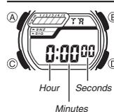
The countdown timer can be set within a range of 1 minute to 24 hours. An alarm sounds when the countdown reaches zero.
